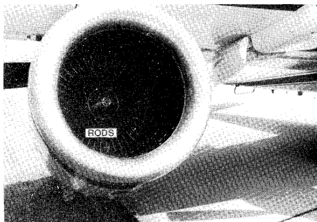
Fig. 2 JT15D inlet with rods installed.
